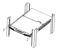
2. While the first person still holds the KL1116 in place, the second person slides the L brackets into the KL1116's side mounting brackets from the rear until the bracket flanges contact the rack, then screws the L brackets to the rack.
